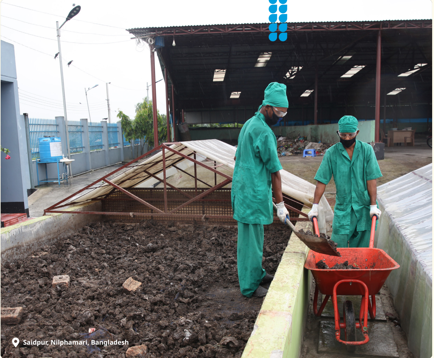
Faecal sludge management plant operator shifting sludge from drying beds.
