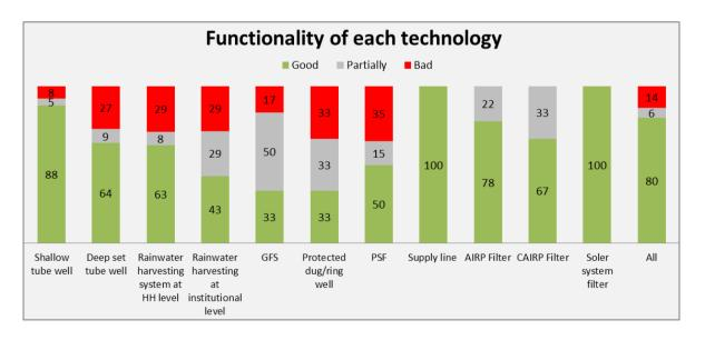
**Functionality of WPs:** About 80% of the WPs surveyed were functioning well, 6% partially and the remaining 14% were non-functional. Higher rates of non-functioning WPs as compared to average were reported/ observed for DTW (27%), RWH (29%), Ring/Dug well (33%) and PSF (35%). The
