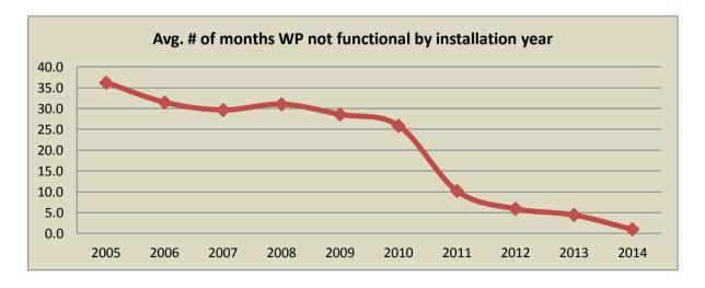
Inclusion of long time non-functional WPs specially those in 2005-2009 into this calculation appears to have resulted in the above higher non-functionality estimates. However, the non-functionality of WPs appears to be highly prevalent even at present while we see the incidence of discontinuity for more than 2 days in the last 2 weeks. This is about 15% combined all. Such estimate is especially
