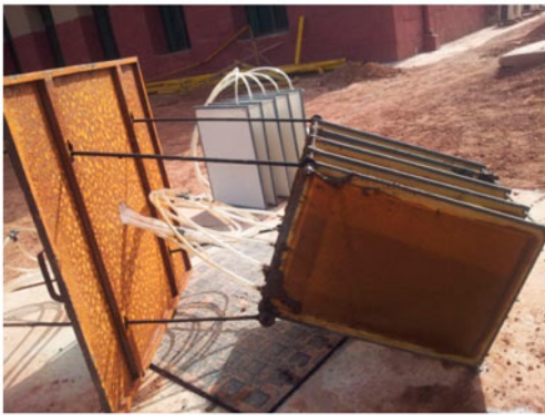
Fig. 2. Membrane module along with manhole cover.
