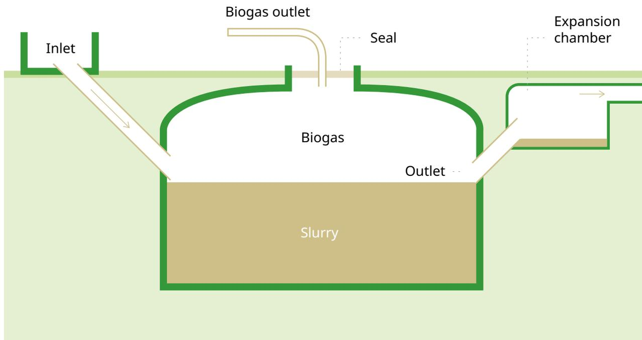
**Fig 4: Anaerobic biogas reactor**
