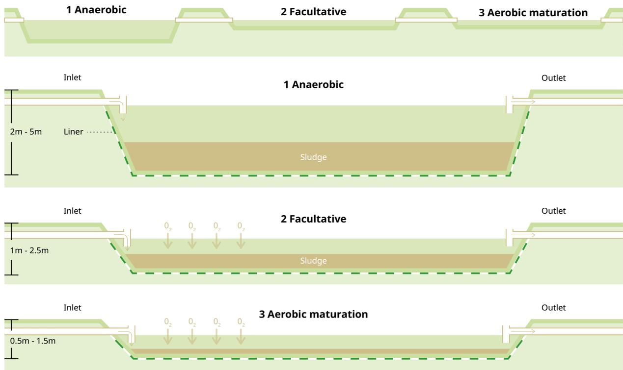
**Fig 3: Cross-section of waste stabilisation ponds**
